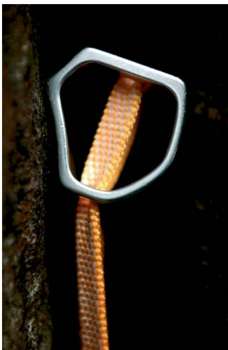
Well placed hex, but crack is flaring below Photo – BMC
