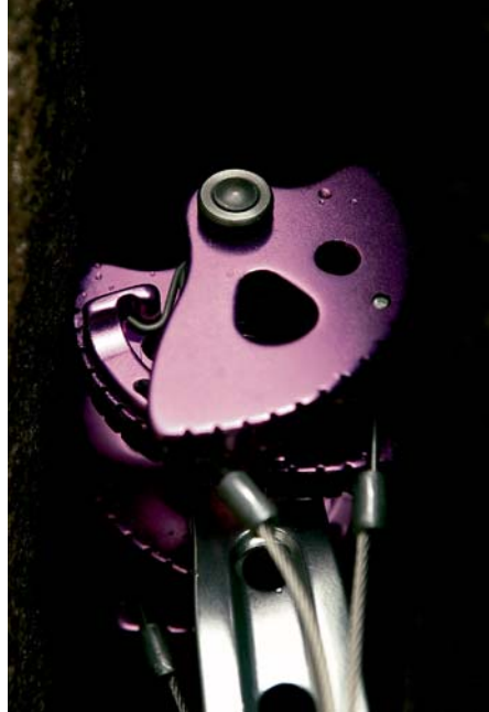
Poorly placed – over cammed
